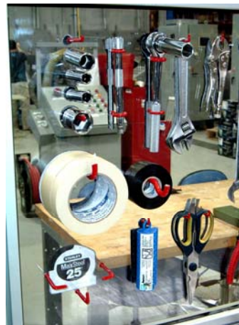
Figure 2: Look closely here is a simple 'shadow board' on Lexan
